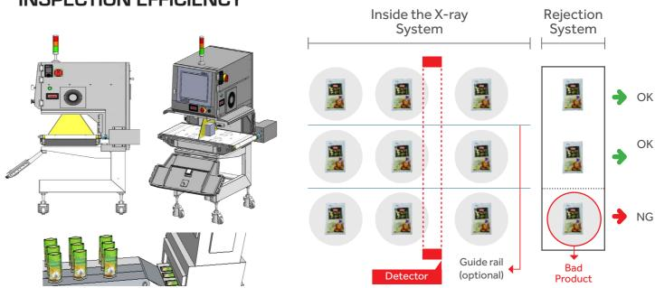
Single packaged products are controlled simultaneously in 2~4 rows. Rated products in each row and sorted out.
