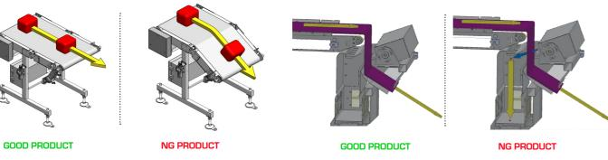
Pusher It sorts products on a conveyor using an air-driven device. It is suitable for Shuttle The belt on the rejector is expanded during the rejection to let NG products rejecting heavy items such as cardboard and kraft paper products fall. It is suitable for unpackaged pet food and sticky Bulk products. Flipper It is a general purpose system, appropriate for thick products.
